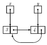
The combination of \* and  $\mapsto$  leads to remarkably simple axioms. In particular, when an assertion of the form  $P*(x\mapsto a,b)$  holds prior to a component assignment x.1:=z we know that the assignment cannot affect P, and so  $P*(x\mapsto z,b)$  will hold on conclusion. The logic of pointer swing is treated in a local way that mirrors the intuitive operational locality of assignment.
